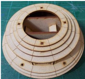
Attach the last two rings – again slotting the upper one onto the lugs on the support posts.
