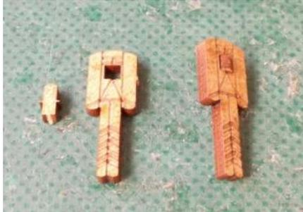
The guns are formed from the pieces on the left. When inserted, the rounded end of the lug will extend through the gun (see right of pic)
