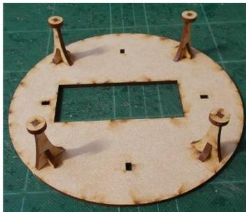
Glue the support legs to the underside of the base as shown above.
