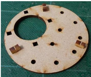
Turn the cap over and glue its lugs into place.
