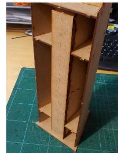
Glue the windows strip into place with the widest blank at the bottom. The strip will touch the base and have a small gap at the top.
