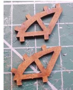
There are two types of dome support – one with a lug at the top and one without.
