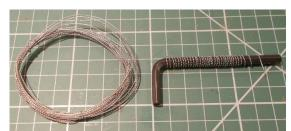
Remove a length of wire from the spool provided. Each long base uses 71cm of wire, each short base uses 36cm of wire.
