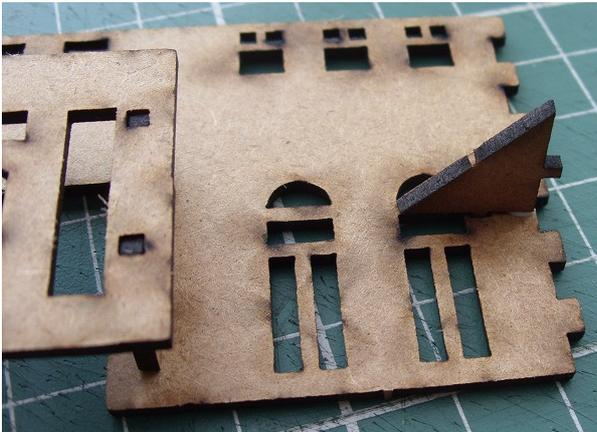
At the same time, glue a triangular bracer to the back of the long sides at each end. Leave these to dry.
