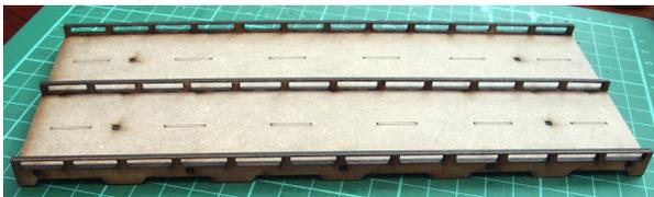
Then glue the side sections and central barrier into place – again using the lugs/holes provided.
