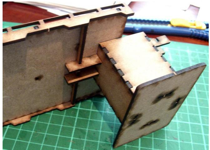
To attach the support columns, simply slide the cross support into the notches in the support column arms. We suggest that you **do not** glue these into place as it will make set-up and storage easier.
