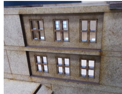
As with the inner walls, the etched lines will align with the edges of the openings.
