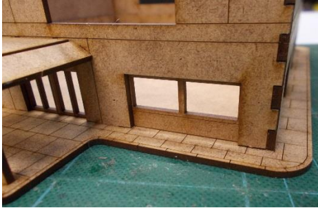
The etched lines on the inner walls will align with the edges of the openings.
