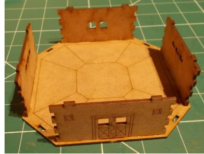
Glue the walls to the base so that the etched details face outwards (see pic)
