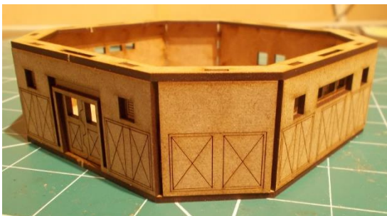
These glue over the top of the inner walls so that the doors / windows can be seen through the gaps. (see pic above)
