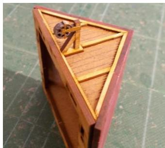
Take the pulley piece from the sprue and glue it into place.
