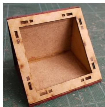
Glue the roof plate into position.
