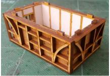
Starting with the door framework, glue this into place aligning the window supports into their spaces.
