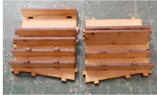
Glue the connectors to the main supports – the wider connectors being the ones closest together.
