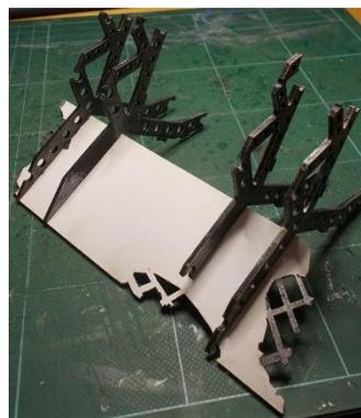
Attach the gantry supports to the back of the hull section as shown above.
