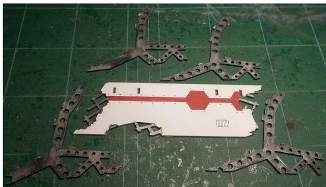
Take the lower hull section and the four gantry supports.
