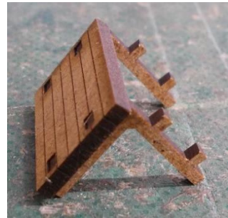
Glue the two supports to one side of the cover. As the pieces are thin, only apply pressure to the lugs.
