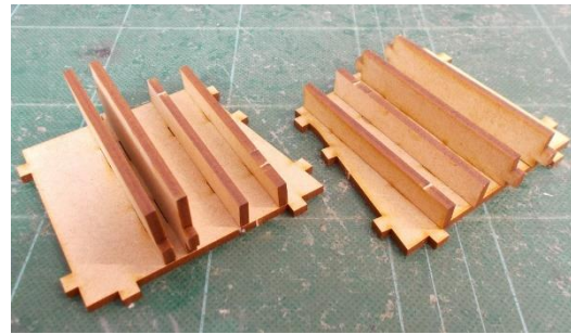
Glue the connectors to the main supports – the wider connectors being the ones closest together.
