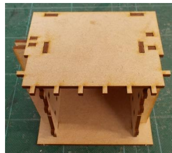
Add the walkway section, gently slotting each lug into the corresponding hole.
