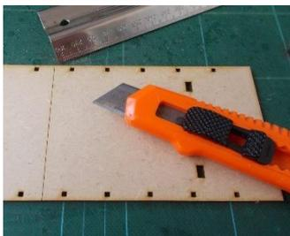
Using a sharp knife and metal ruler, cut the side platform along the line.
