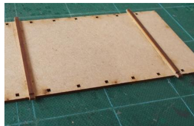
Attach the supports under the platform using the holes / lugs provided.
