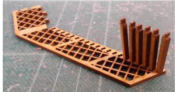
Starting from the bottom, glue the steps to the side piece as shown.
