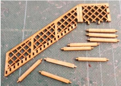
Remove one of the step side pieces and the corresponding number of steps from the sprue.
