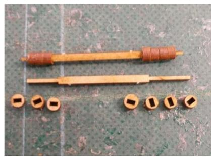
Each support is formed from the pieces at the bottom of the picture.
