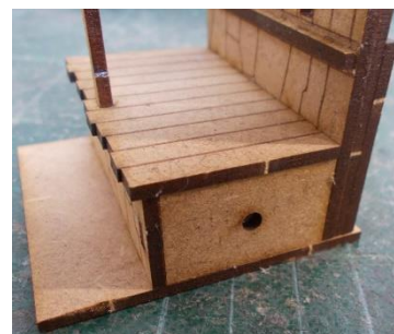
Add the end plate to each side of the model. Note: the holes will accept 2mm diameter neodymium magnets (not supplied)
