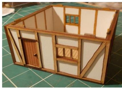
Then take the insert sections from the sprue and glue them into the spaces in the framework. Note the insert pieces for each wall are in their relative positions on the sprue.
