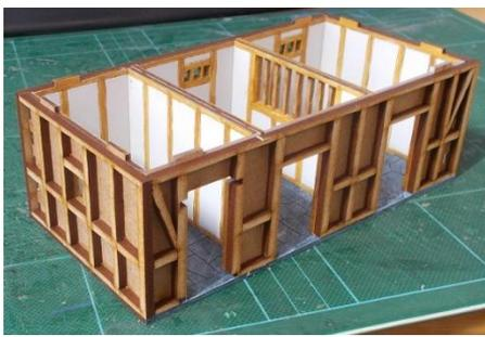
Take the frames shown above. Starting with the doorway, glue the frames into position. They will align on the left and extend out by around 3mm on the right.
