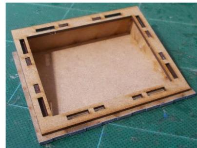
Glue the roof plate into position.
