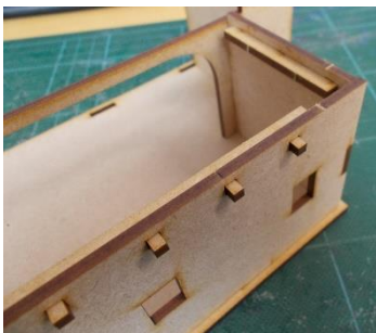
Glue the supports into place, inserting them through the back of the wall.
