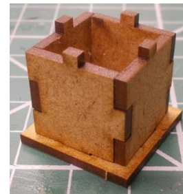
Glue the walls to the base as shown above.
