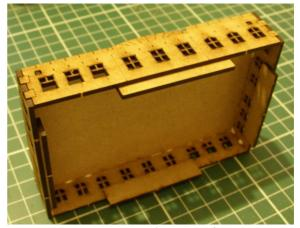
Apply glue to the edges of the roof and attach the walls to it using the lugs provided (etched detail outwards).
