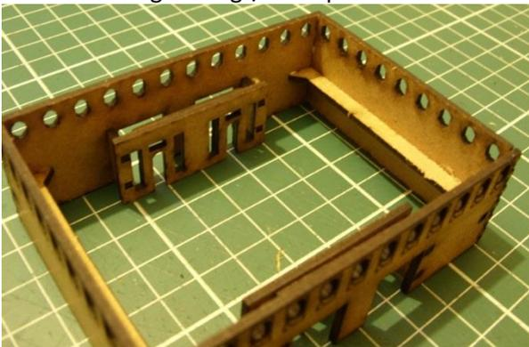
Glue the walls together to form a hollow box structure. Leave these to dry.
