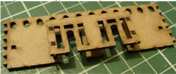
Glue each doorway to the **back** of the long sides, using the lugs/holes provided.
