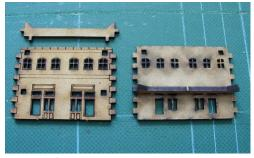
Take each of the wide wall sections and its brace piece (shown on the left). Glue the brace to the rear of the wall (shown on the right)
