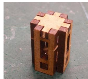
Glue the end cap in place.
