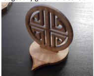
Glue the smaller disk below the larger one, aligning the slots and then push the upright through to secure them in place.
