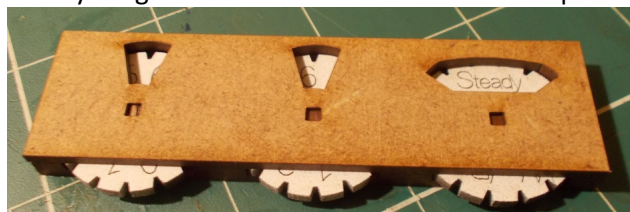
Carefully glue the top plate into position (making sure no glue gets onto the dials), aligning the axles with the holes provided as shown above. Leave to dry.
