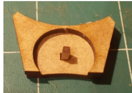
Glue the axle to the back plate, then glue the surround in place.
