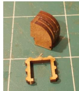
Glue the pieces together to form a 4-layer sandwich, ensuring those with the corner cut-outs are on the outside.
