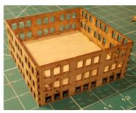
Glue the walls to the base as shown, aligning them using the holes / lugs provided.
