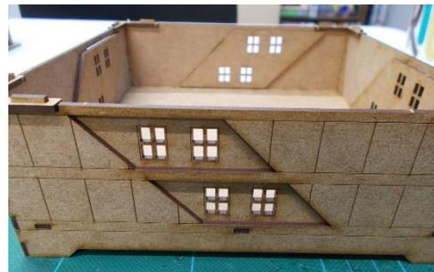
The etched lines will align with the edges of the openings.
