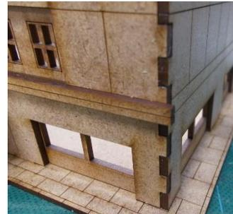
Glue each one in place – it aligns with the left hand edge and will extend out by 2mm at the right hand edge.
