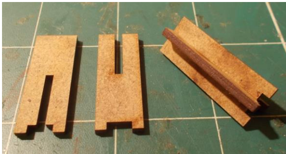
Each support is formed from the two pieces on the left. Slot them together as shown on the right.
