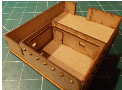
Glue the door behind the opening and attach the supports by pushing the lugs through the holes in the walls so that they stick out as shown above.
