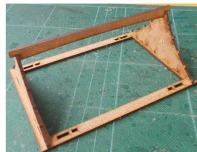
Place (do not glue) the side sections into the roof plate and glue the beam between them as shown.
