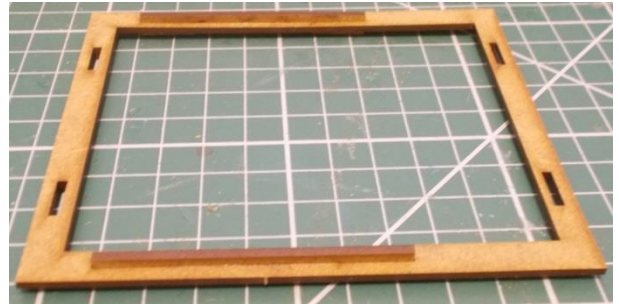
Glue the support bars through the holes in the roof plate.
