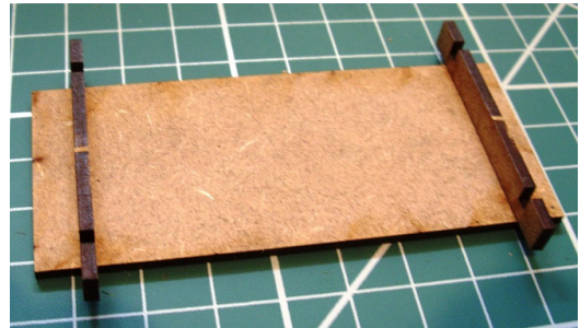
Glue the short supports in position (as shown) on the underside of the base.
