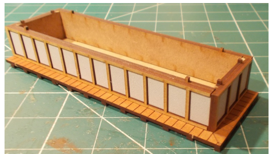
Glue the wall panels into place.
