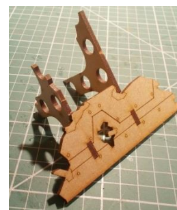
Glue the supports to the back of the "wall" using the lugs / holes provided.
