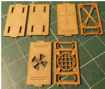
The three wall types with their inner piece (left) and outer piece (right) (Join, Girders, Fan)
