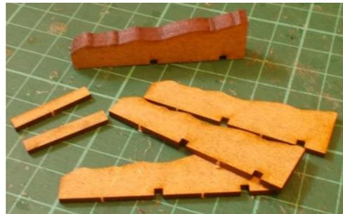
Take the contour sections and glue 3 or 4 together ensuring the notches align.
