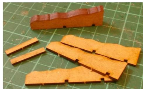
Take the contour sections and glue 3 or 4 together ensuring the notches align.
