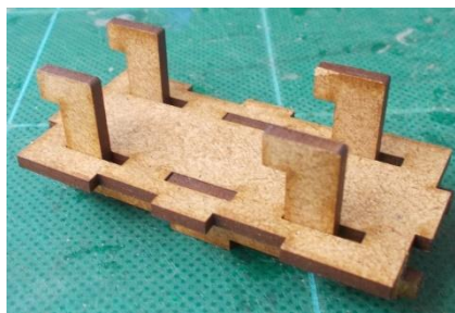
Glue the two hooked pieces through the back plate, ensuring the hooks all point in the same direction.
