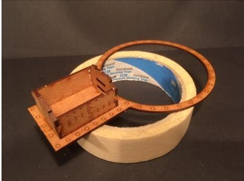
Glue the four pieces into the plate section ensuring that the slotted end plate for the engine is at the end with the loop. You will need to elevate this section as there are pegs that protrude through.
