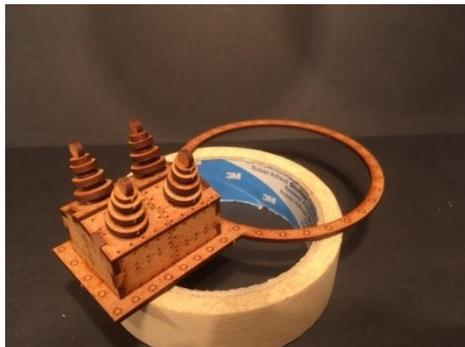
Glue the four power coils into place on the top of the engine.
