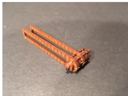
The first isk on the pin should be the smallest. Then the first chain, then two cogs, the next chain and lastly three cogs.
