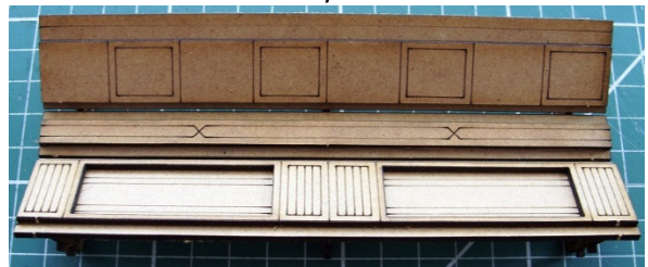
Glue these into position on the wall (NB: There are lines inscribed on the wall to help you position these). Leave to dry. Ensure the decorative pieces do not extend over the ends of the wall as this will make linking corridor sections together quite tricky.
